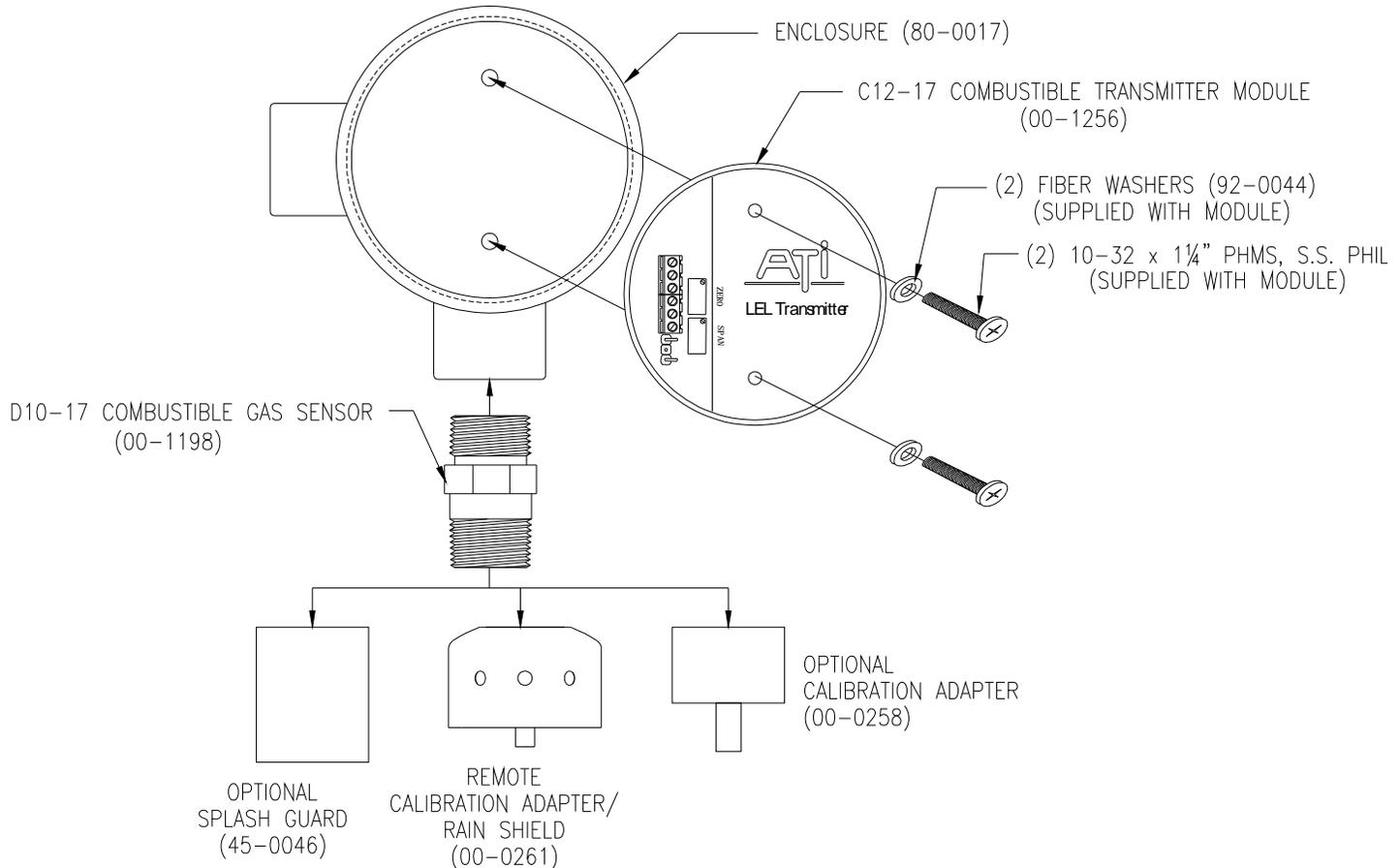
**Figure 10 - Standard Combustible Transmitter Exploded View (ATI-0146)**
