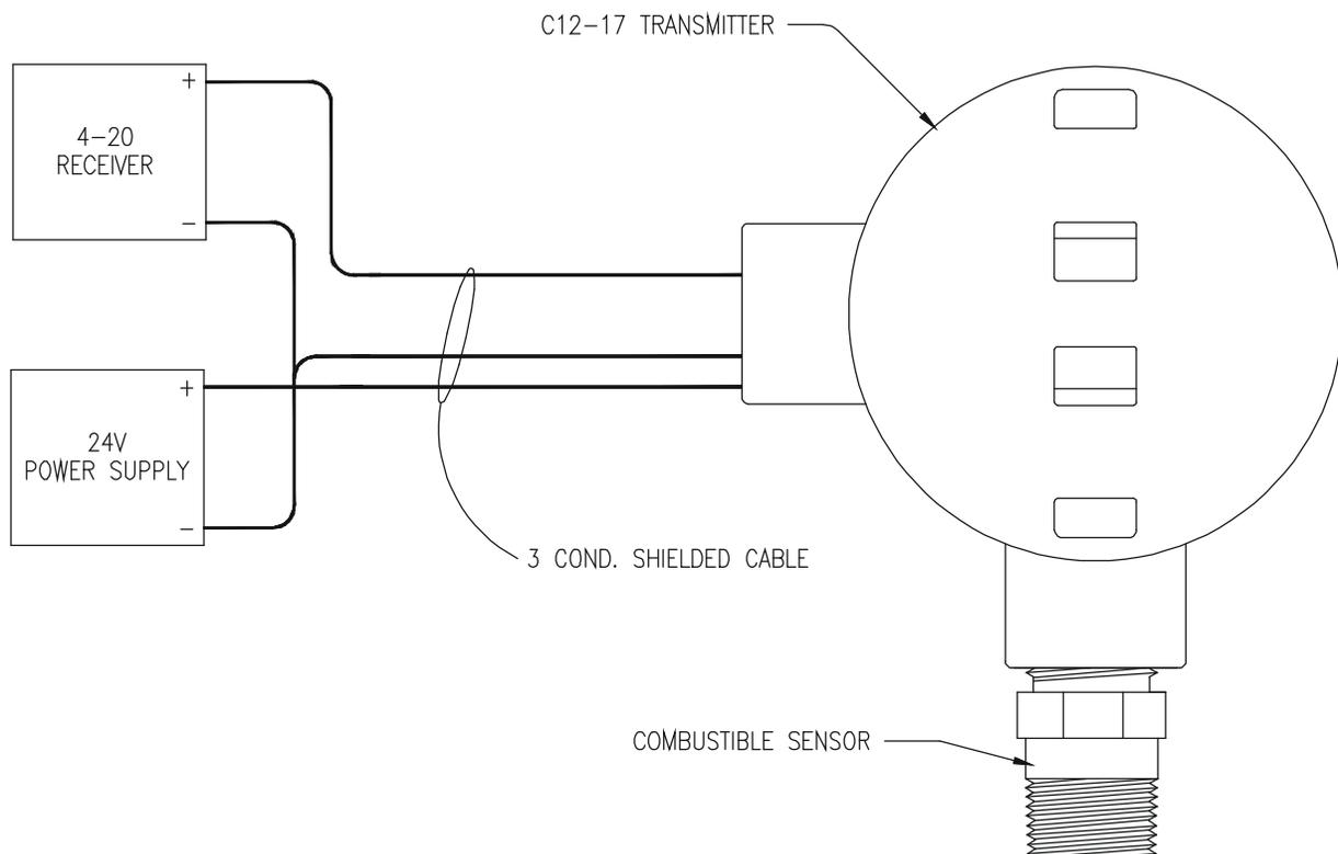
**Figure 1 - Typical System Diagram (ATI-0145)**
