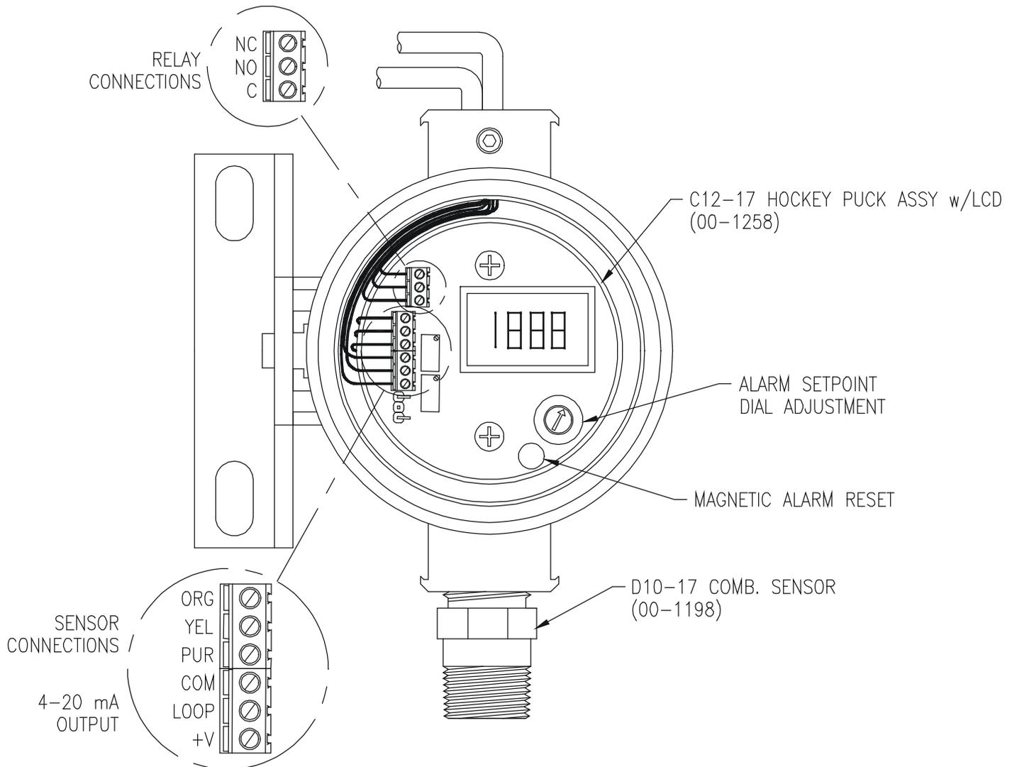
**Figure 9 - Transmitter with Display Customer Connections (ATI-0570)**
