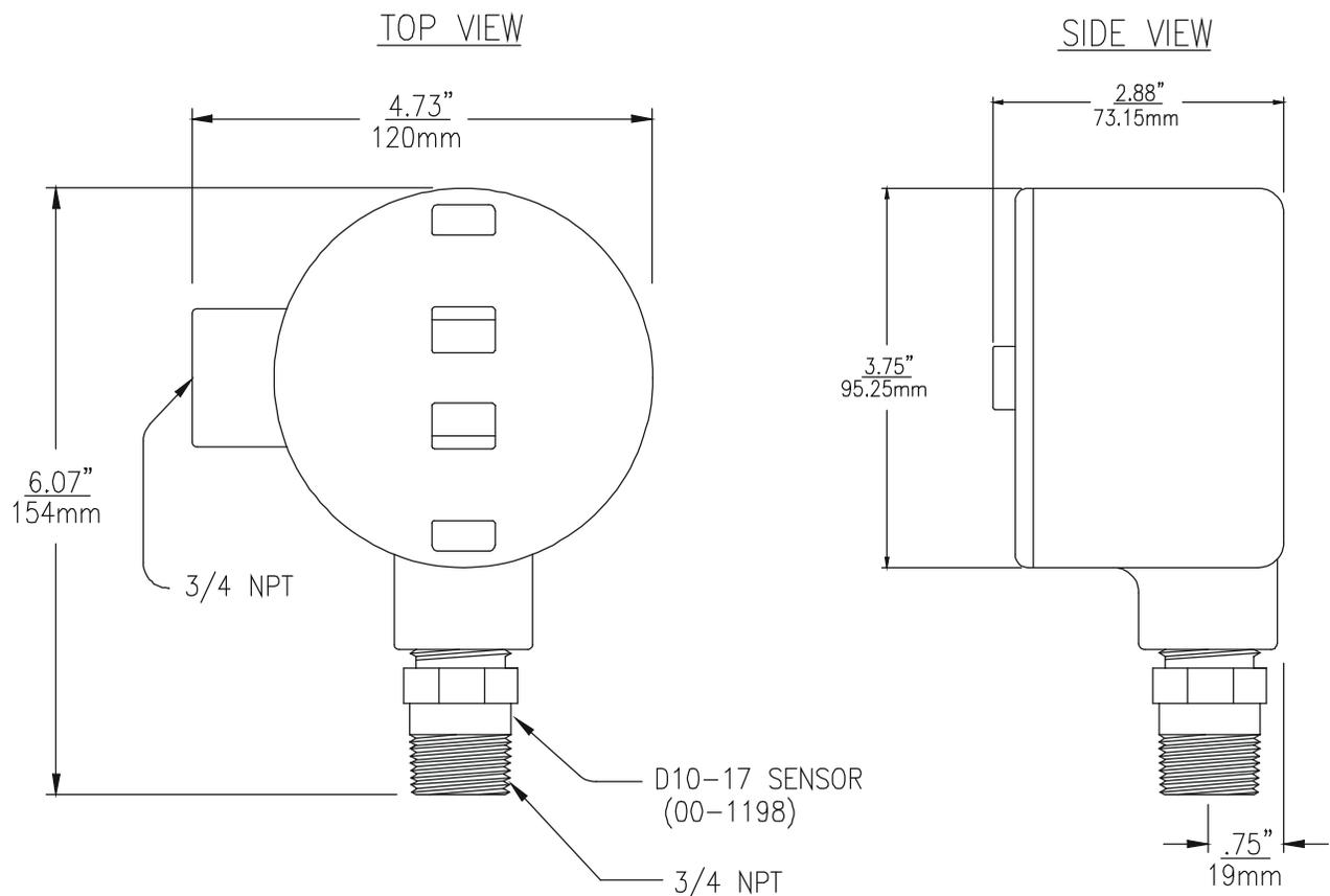
**Figure 2 - Combustible Gas Sensor/Transmitter Dimensions (ATI-046)**
