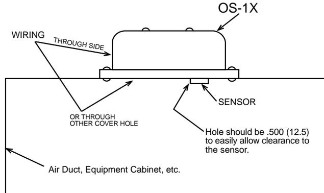
**CAUTION!** Avoid excessive touching of the inlet end of the sensor and keep it free from chemicals, lubricants, dust, water, etc. Do not use silicone caulking compound or RTV near the sensor.
