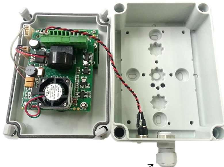
Cable gland for RS232 or RS485 connection
