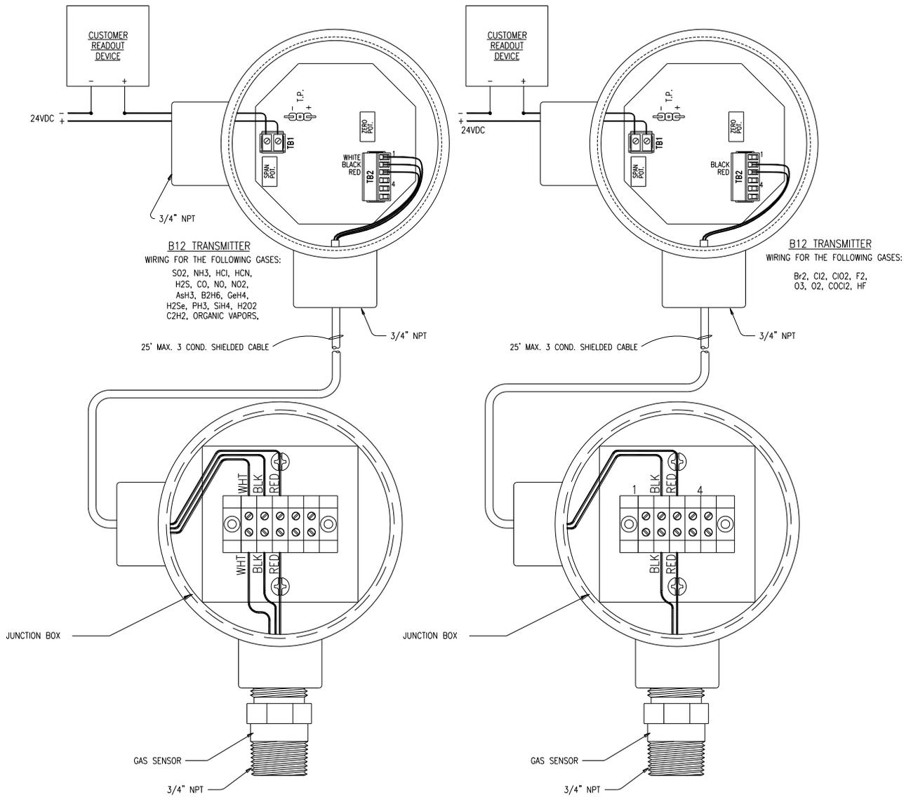
**Figure 8 - Electrical Connections - C10 Dual Condulet Sensors (ATI-0101)**
