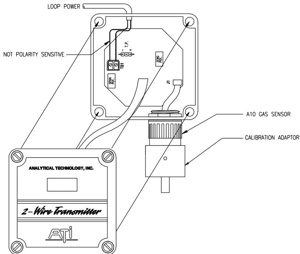
**Figure 11 - Transmitter Controls & Test Points (ATI-0205)**
