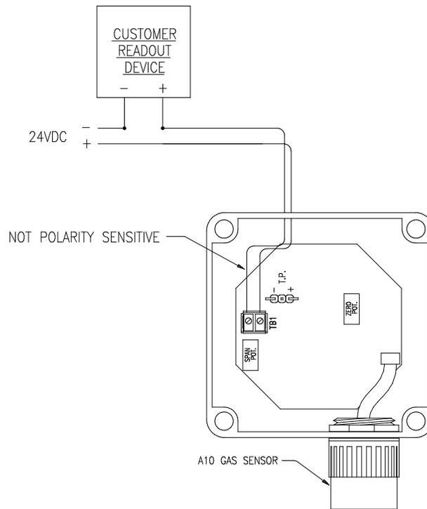
**Figure 5 - Electrical Connections - Standard System**
