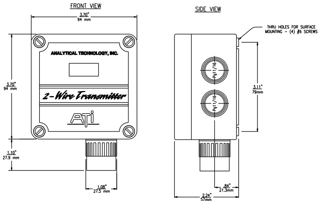
Figure 1 - Series B12 Nema 4X Transmitter Dimensions
