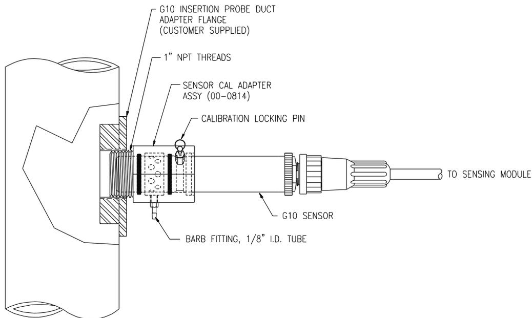
**Figure 12 - Duct Mount Sensor Calibration (ATI-0299)**
