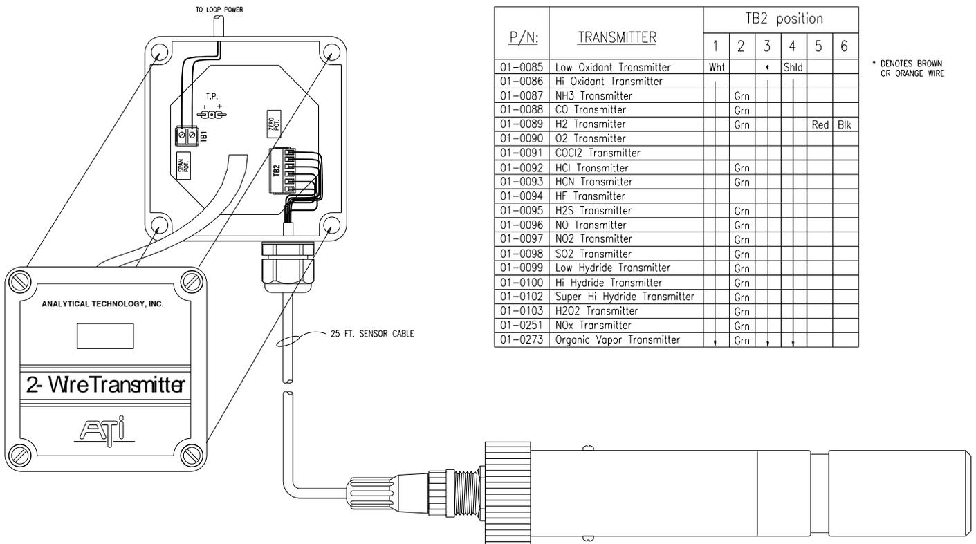
NOTE: All conductors on cable only used on H2 sensors only, the RED and BLK conductors can be removed from cable for all other gas applications.
