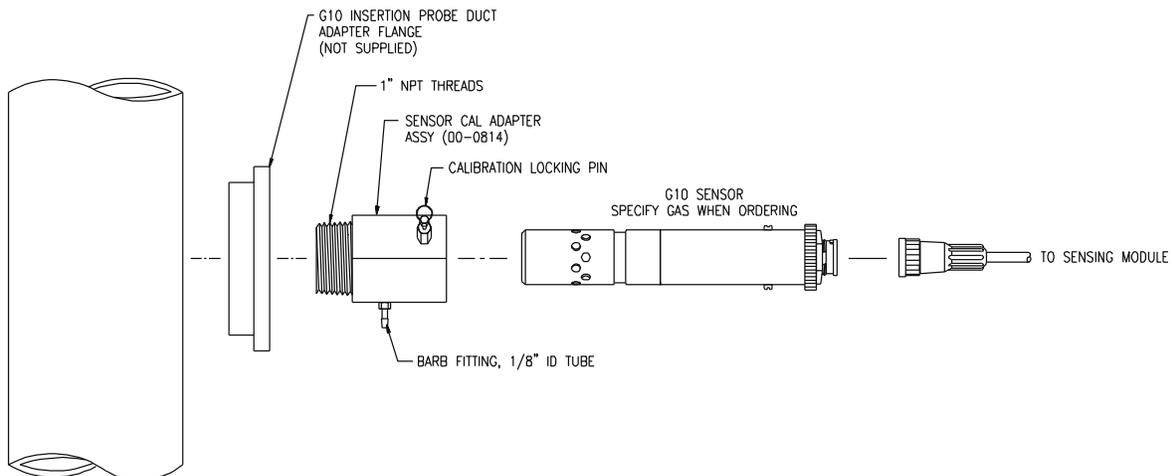
**Figure 4 - Duct Mount Sensor Installation (ATI-0298)**
