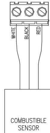
**Figure 4 - Sensor Connections to Transmitter (ATI-0144)**
