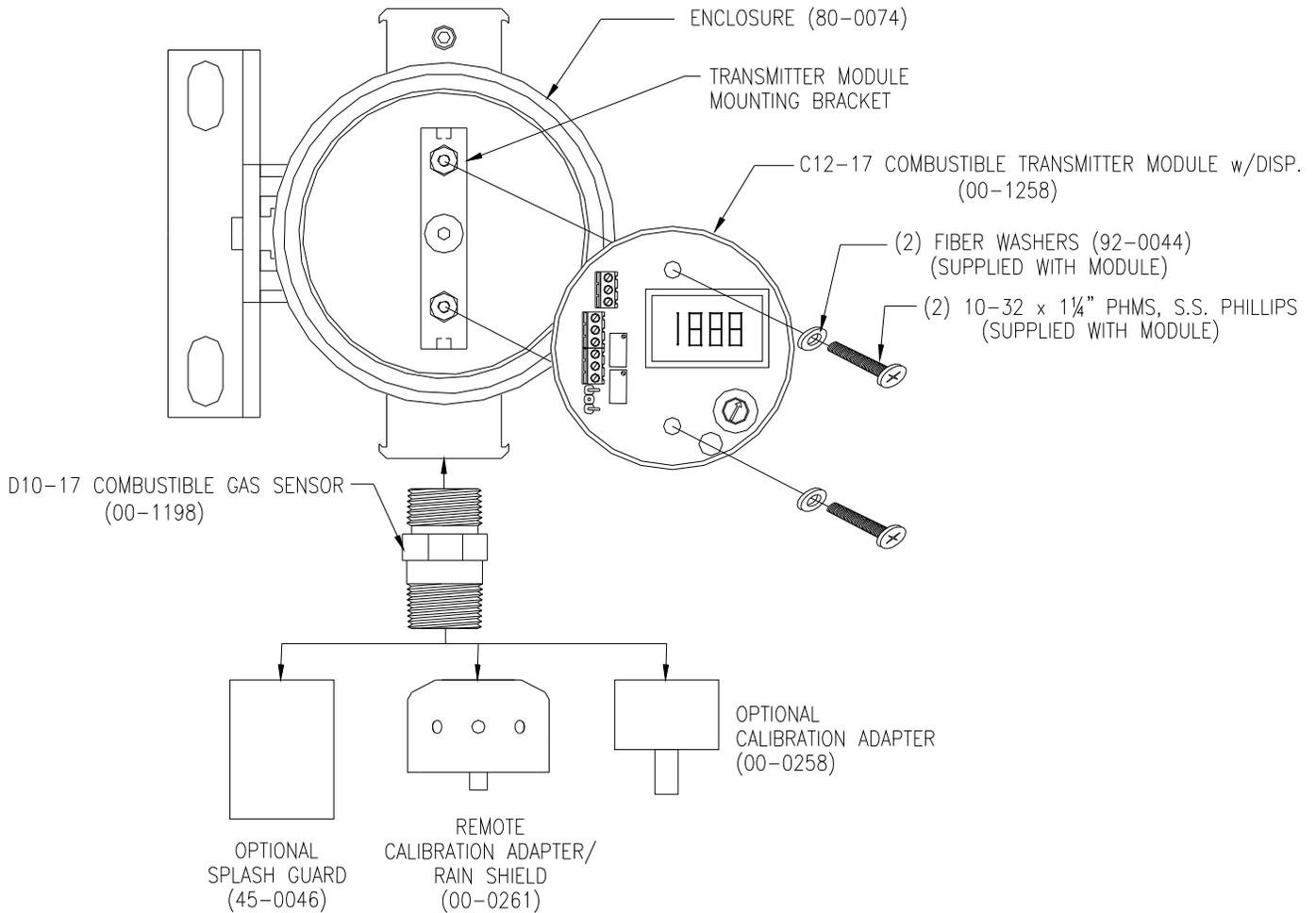
**Figure 11 - Standard Combustible Transmitter Exploded View (ATI-0571)**
