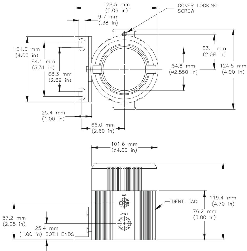
**Figure 8 - Enclosure with Display Dimensional Drawing (ATI-0569)**
