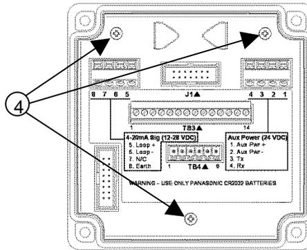
4. Remove the Terminal PCB by pulling straight up, to expose the CPU PCB (5).
