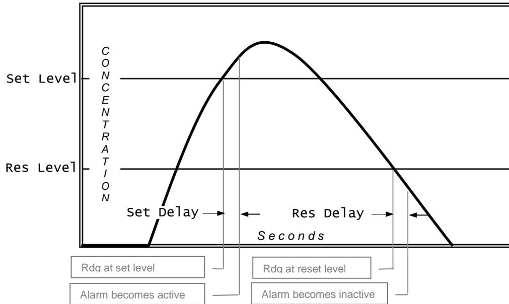
**Figure 53. High Alarm Operation**
