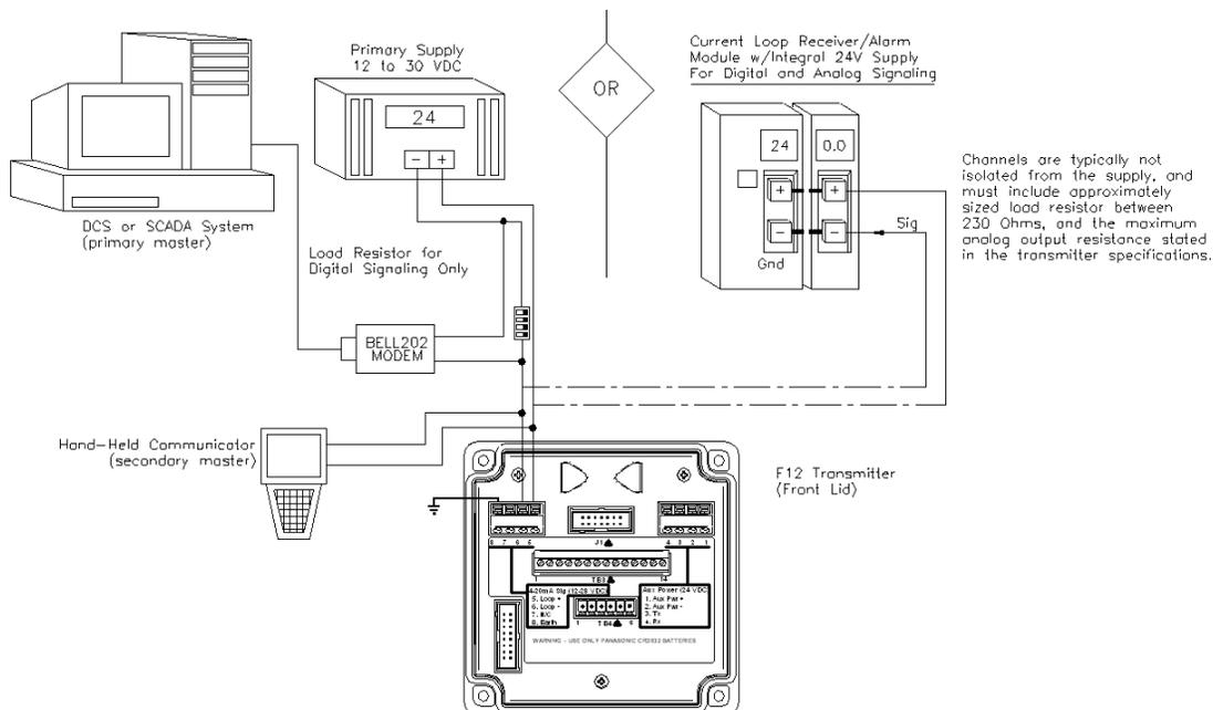
**Figure 17 - HART Point-to-Point (2-Wire)**
