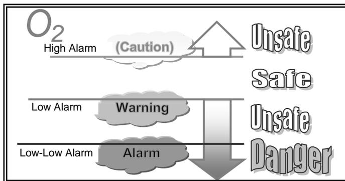
Figure 52. Oxygen Deficiency Alarms
