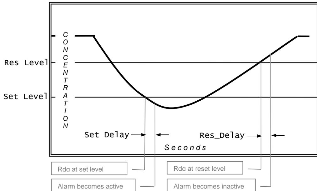
**Figure 54. Low Alarm Operation**
