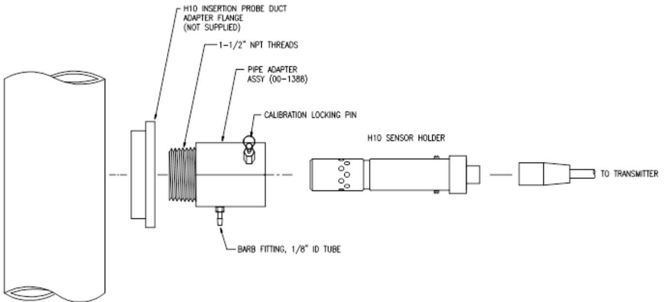
**Figure 12. Duct-mount assembly**
