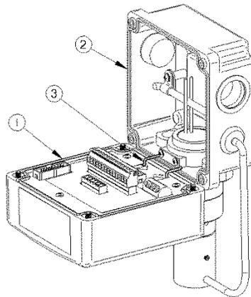
3. Remove the Internal Shield by removing the three screws (4)
