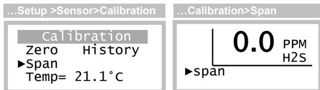
Figure 40. Sensor Span Cal. Menus
