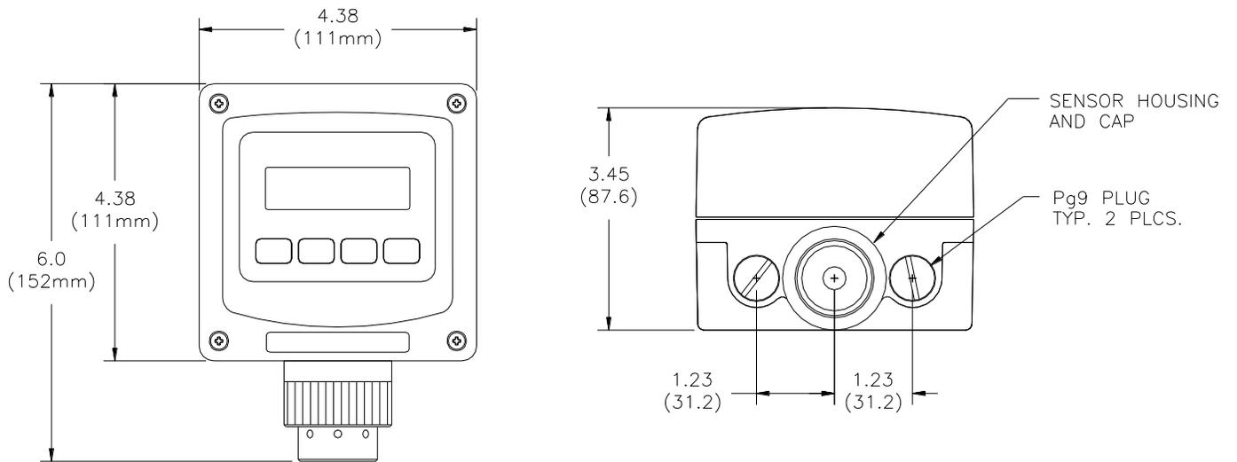
**Figure 4. Enclosure dimensions, (standard)**
