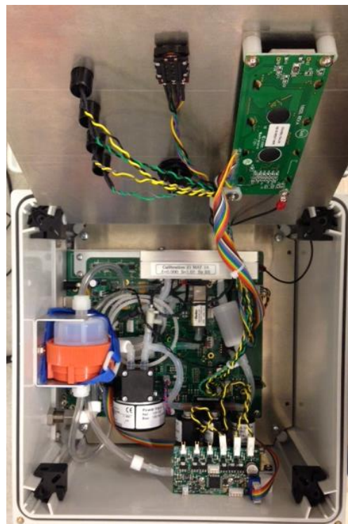
Figure D-7. (a) Side View of the Model 106-M-MC6 Multi-Channel Ozone Monitor. (b) Top inside view of Model 106-M-MC3, with filter installed (see Figure D-5 for component labeling).
