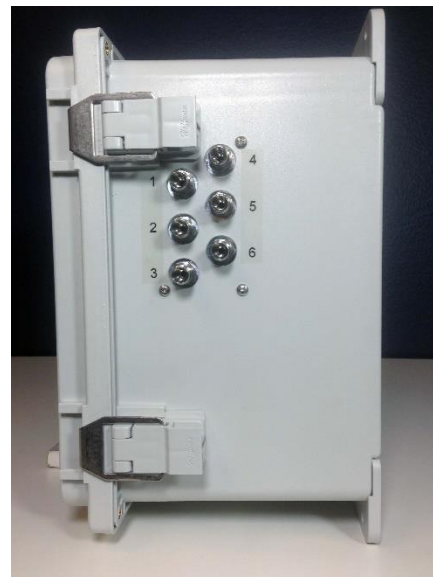
Figure D-4. ¼-inch Swagelok inlets on the side of the 6-channel instrument.
