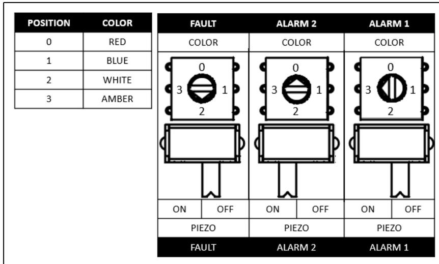
Figure 22: LED and Buzzer Selection Panel
