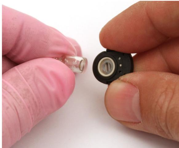
**Figure 27: Reinstalling the Electrode Lamp**
