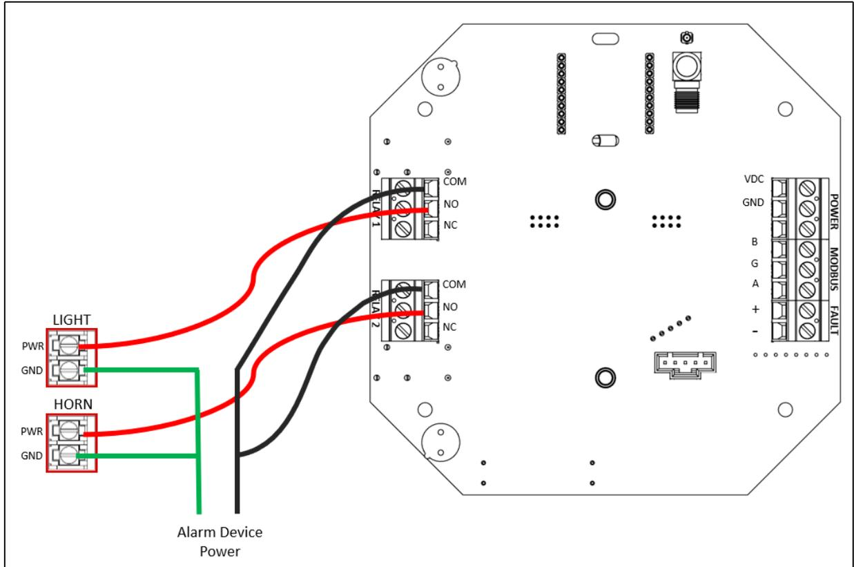
**Figure 18: Relay Wiring**
