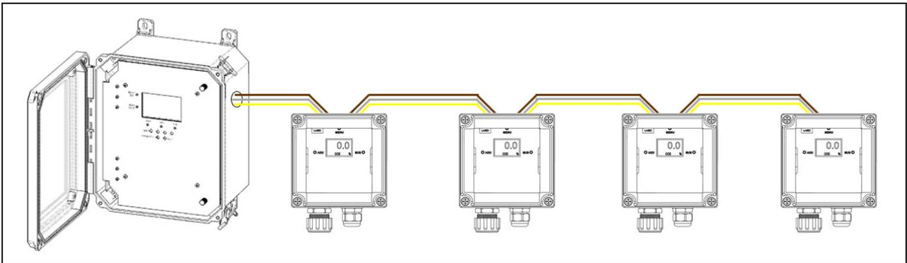
The signal wire of each unit is run to the signal terminal of the neighboring sensor. With each device connected to the previous device via the signal wire, a “chain” is created, with the first device in the chain directly connected to the controller.
