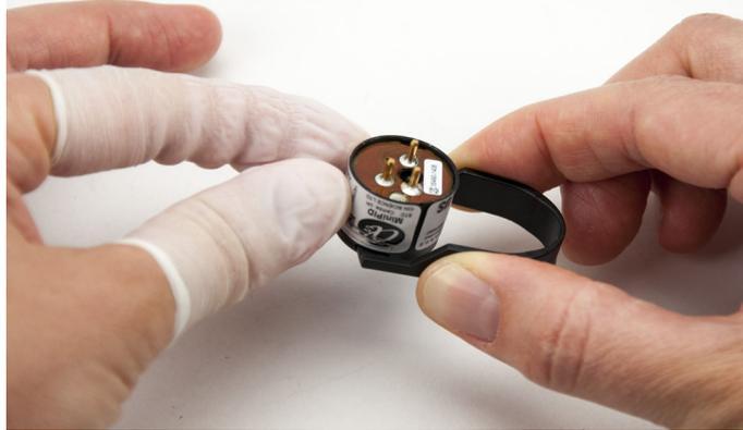
**Figure 30: Using Removal Tool**
