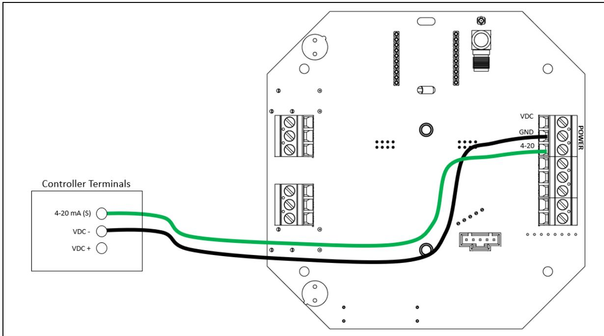
Figure 15: 4-20 mA Wiring for AC-Powered Relay Version
