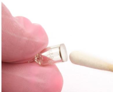
**Figure 26: Polishing the Electrode Lamp Window**
